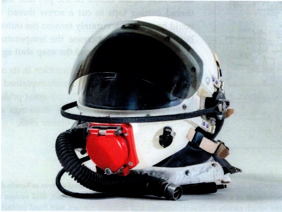
Taylor RAF Partial Pressure Helmet Notice the red access door for refreshment or if air sick.
